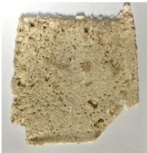
60% crushed shell + PLA
