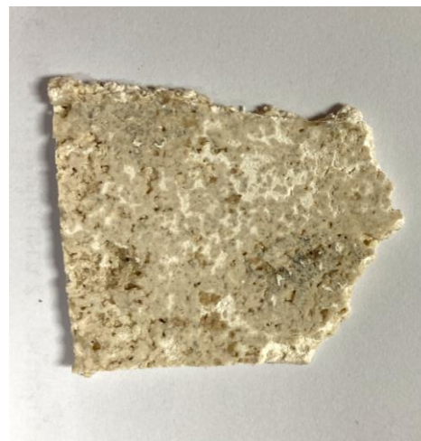
70% crushed shell + PLA
