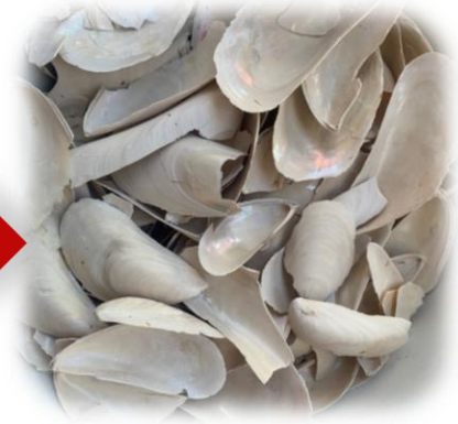
Bake at 300°C for 3 h to remove organic component
