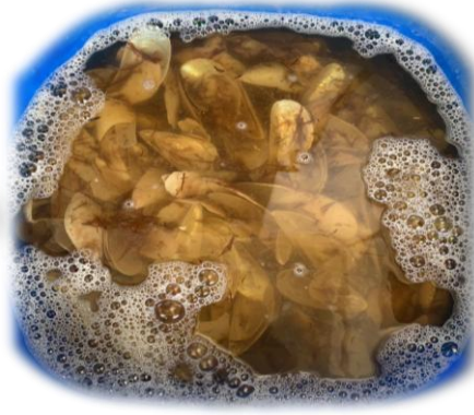
Immersion in 1 M KOH solution for 14 days to remove protein
