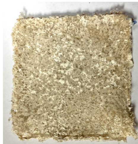
50% crushed shell + PLA
