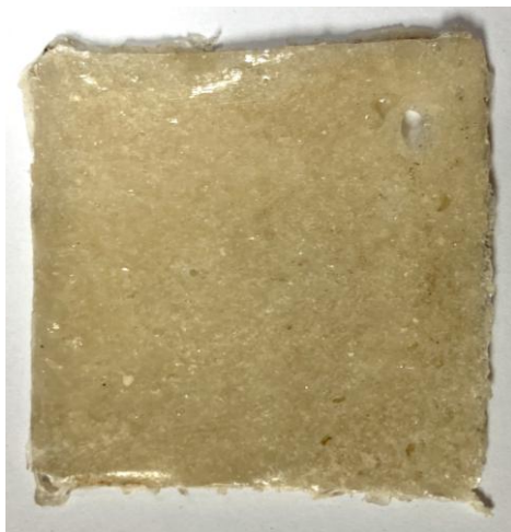
10% crushed shell + PLA
