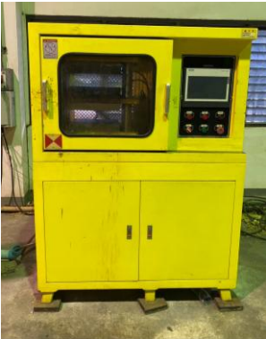
Forming Bio-CaCO 3 /PLA compound with hot compression molding
